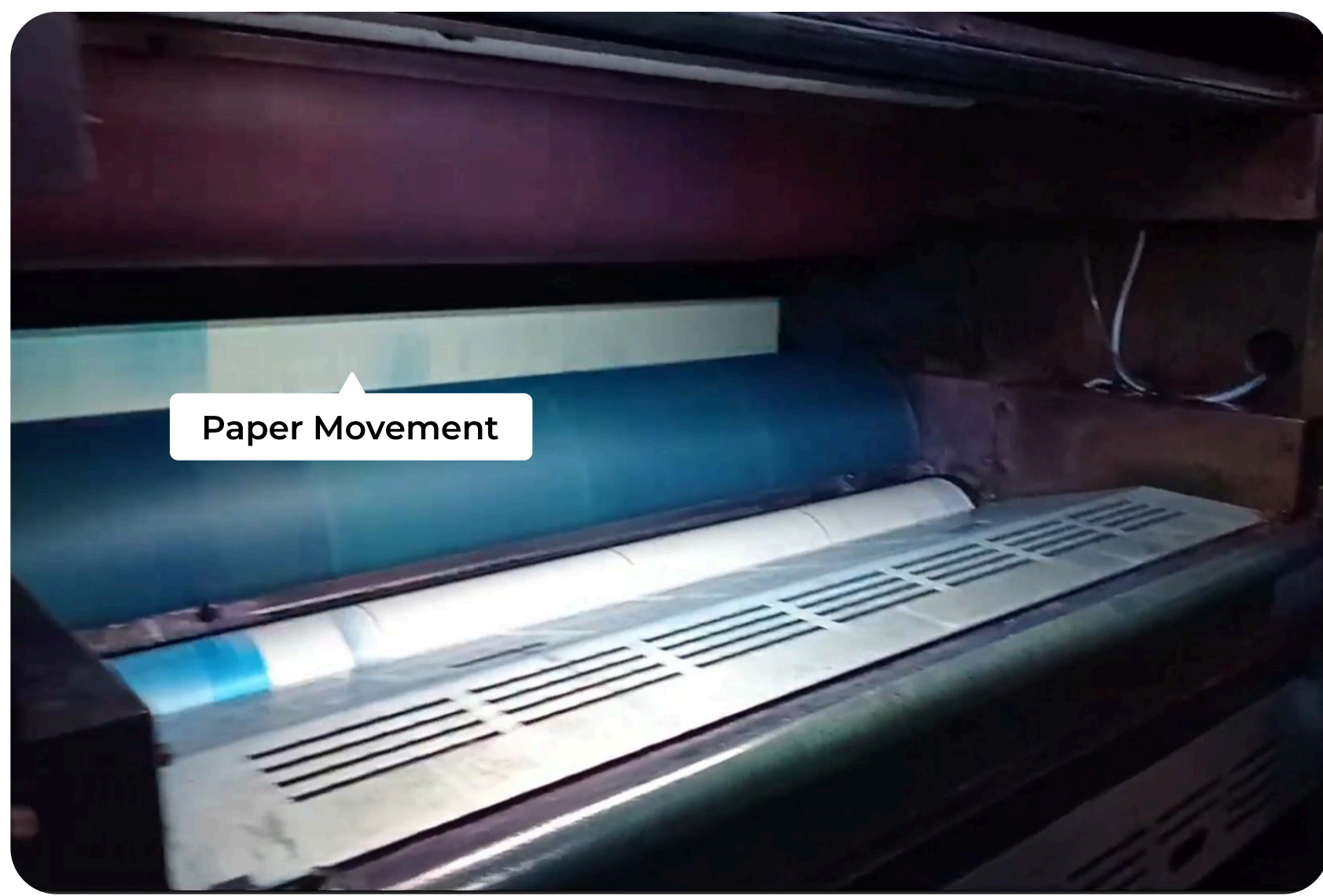
Figure 2(b) Paper Movement Between Unit 1 & Unit 2 Cylinders
